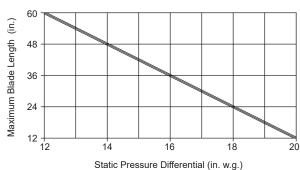
This damper's design at a blade length of 60" has a maximum allowable blade deflection of L / 360 for the static pressure indicated on the chart. At reduced blade lengths, higher static pressure limits can be attained without sacrificing damper operating performance characteristics.
