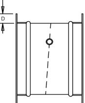
Equal leg angles are available. They are welded to frames at intermittent spacing and caulked between welds. Flange Height "D" varies with damper diameter.
