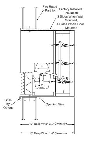
Combination Fire/Smoke Damper • 1½ Hr. Rated • Airfoil Blade • Leakage Class II • 250°F or 350°F Rated • Front Grille Access • Galvanized Steel
