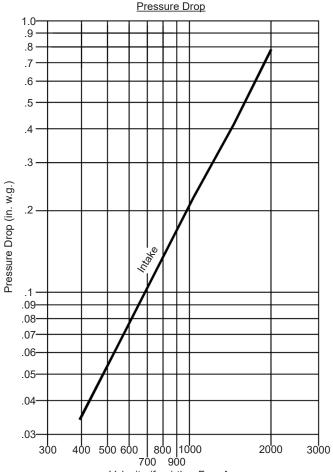
Velocity (fpm) thru Free Area Intake air converted to standard air density. Tested to AMCA Standard 500-L, Figure 5.5.
