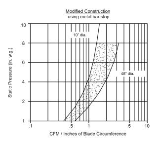
Leakage results shown are based on tests using various damper sizes. The shaded area between the graph lines indicate normal expected leakage range for a standard damper operating conditions and sizes.
