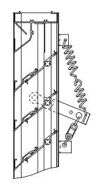
NO. 0-21 SPRING OPERATED WITH FUSIBLE LINK (160° F)
